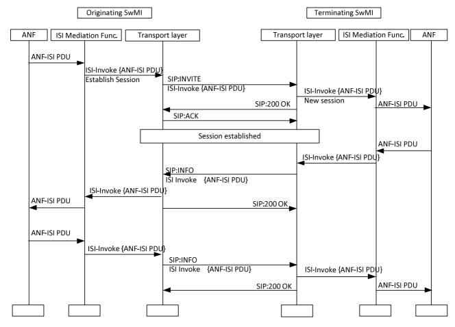
Figure 6.1: Establishment of signalling connection without audio connection
