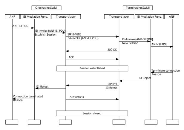
Figure 6.6: Error detected in the ANF during call establishment
